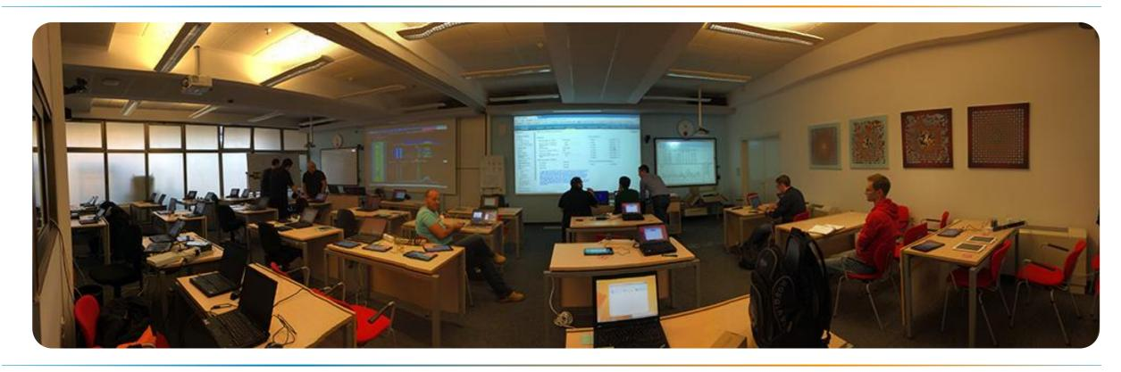
APs were placed outside a classroom separated from the client devices by a single drywall with a measured loss of 5dB. The classroom size was 12 meters (~39 feet) by 10 meters (~33 feet).
